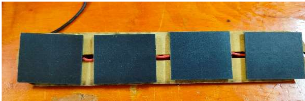
Figure 13 Construction of series array of SM141K10LV cells.
