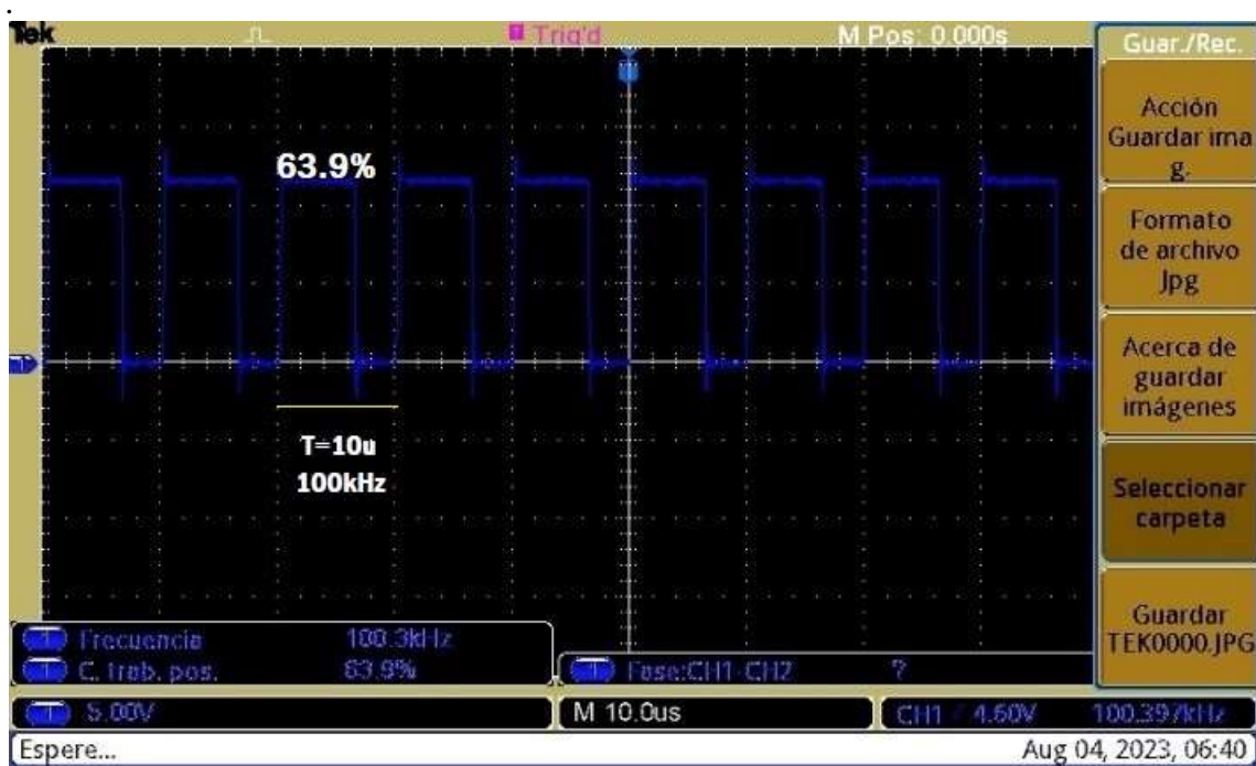
Figure 16 PWM control in elevator mode seen in oscilloscope
